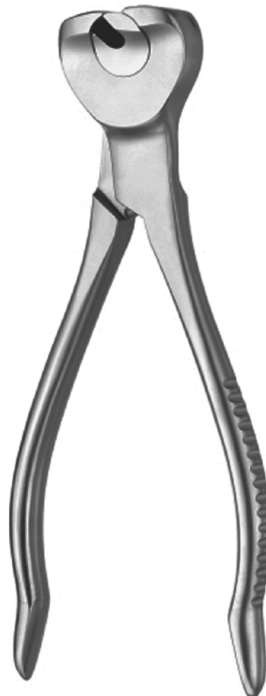
EI-222-16 Wire Cutting Plier For Soft Wires Up to \varnothing 2.2 mm For Hard Wires Up to \varnothing 2.0 mm Overall Length 16 cm (6 ¼")
