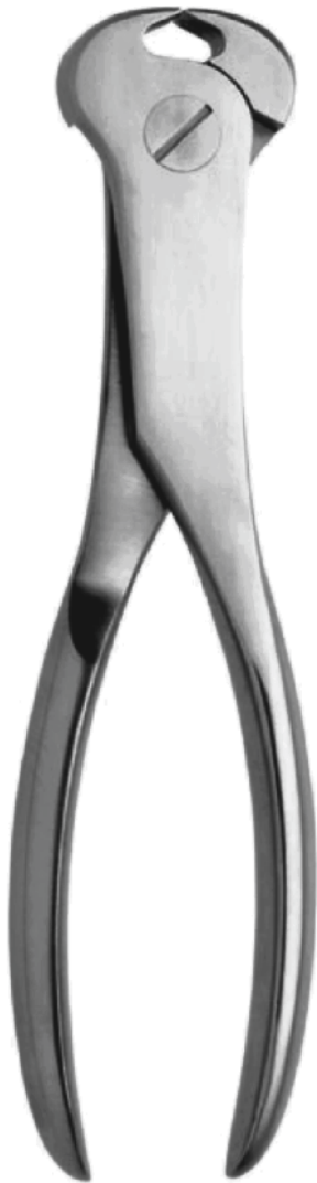
EI-220-18 Wire Cutting Plier For Soft Wires Up to \varnothing 2.4 mm For Hard Wires Up to \varnothing 1.8 mm Overall Length 18.5 cm (7 ¼")
